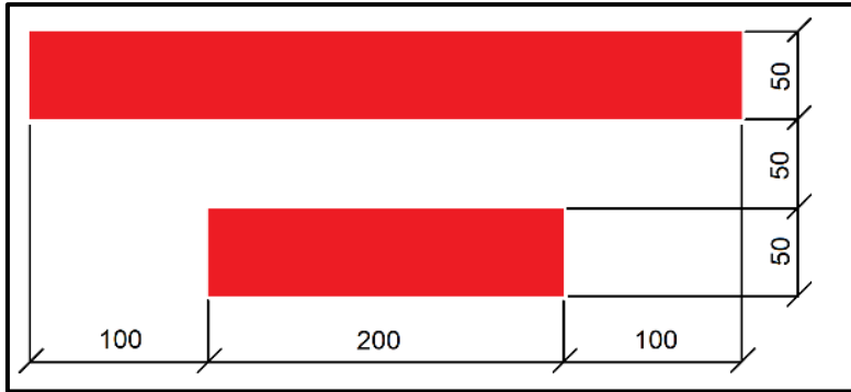
Annex 5: Template for flat strip marking on rock faces (dimensions shown in millimetres)
