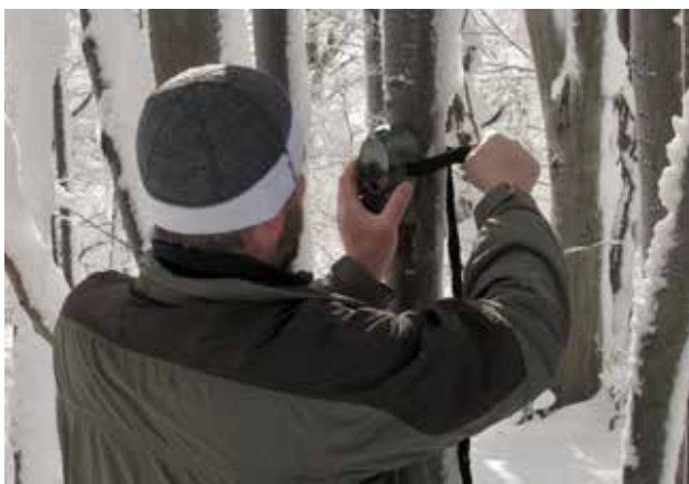
Fig. 12.12 The most common method in assessing the efficiency of fauna passages is the use of phototraps. They must be installed not only in the passage itself, but also in its surroundings. This enables to verify which animals have not used the passage. © Michal Kaláš
